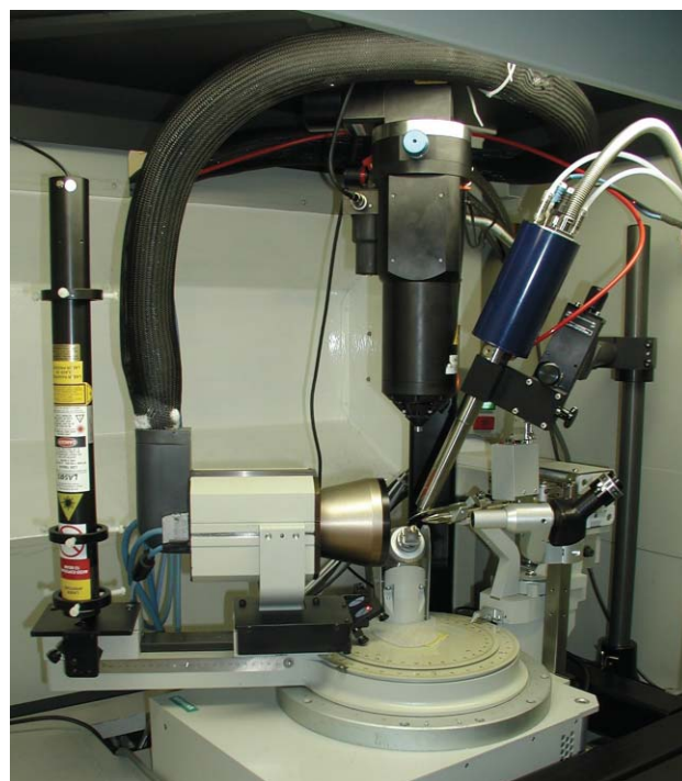
Fig. 6 Bruker SMART-1K CCD area detector diffractometer equipped with both an Oxford Cryosystems Cryostream N 2 and Helix He open flow gas cryostats for low temperature measurements. In addition, a laser is permanently mounted on the goniometer for the measurement of light induced excited states.
